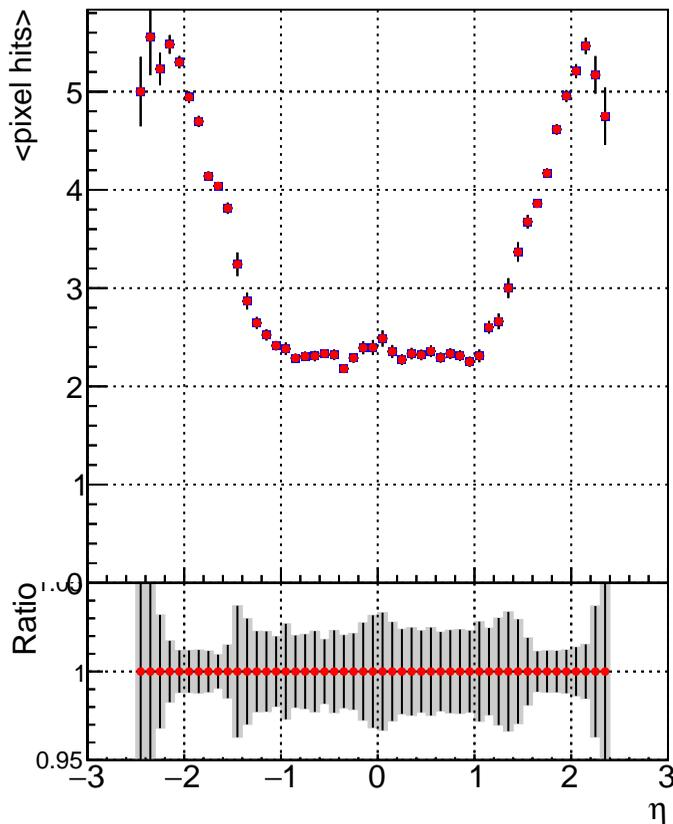
mean # PXL Layers with measurement vs eta
